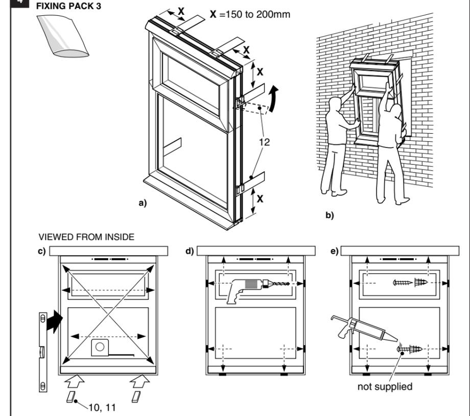
To ensure that the window operates smoothly it is vital that the frame is installed correctly. The frame **MUST** be fitted plumb and square. Check with a spirit level of adequate length, by measuring the frame corner to corner diagonally to achieve an equal measurement, or by using a square. It is also recommended that the window is checked for bowing by using a long straight edge.
