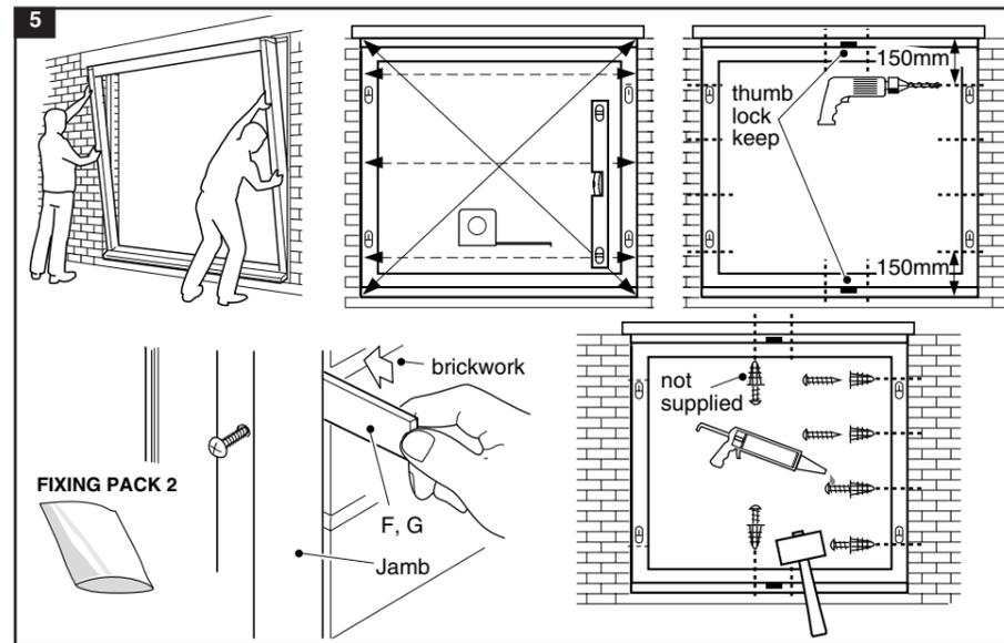
**6** Fill gaps between masonry and the frame; if the gaps are too wide a proprietary expanded P.U. filler or foam rod may be used, prior to finishing with a suitable grade of silicone sealant.
