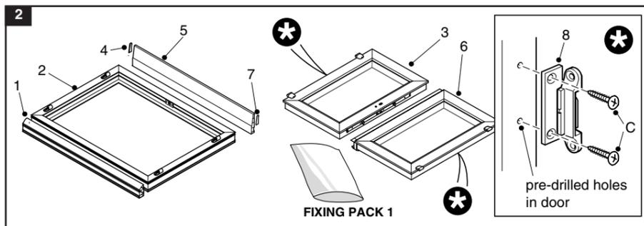
**3** Before fitting the vented head (1), position the outer vent covers to the outside of the head over the pre-drilled slots and fix with the smaller self-tapping screws (H).
