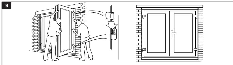
**10** Minor misalignment of the doors can be rectified by adjusting the hinges.
